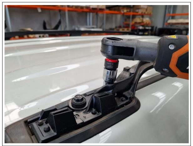
7. Remove the 4x 12mm head bolts securing the front and rear of the roof rail to the roof.
