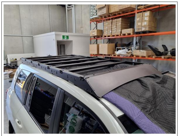
33. With your mate's assistance, lift and place the roof rack onto the roof. Position the rack such that the mounting slots on the rack sides align with the holes on the previously installed mounting plates.
