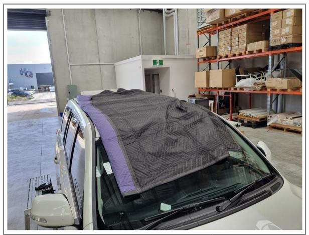
32. Place a soft blanket on the roof in between the roof channels to protect the paintwork while the roof rack is installed.
